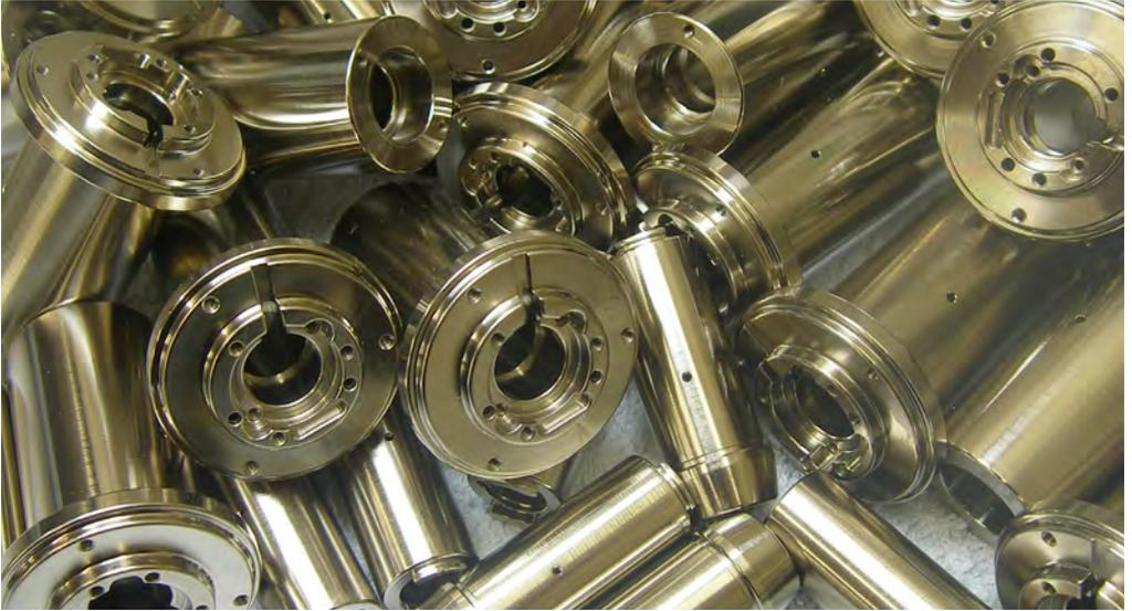
R A Chilton have a long history of copper electroforming. We produce the copper rotors for use in high speed air bearing spindles. The requirement for quality and reliability on these parts, which rotate at incredible speeds of up to 350krpm, is paramount; if they are not exactly right the copper could separate from the rotor and destroy the spindle.
